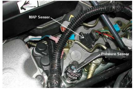
sensor connector into the stock pressure sensor on the engine and the stock engine wiring harness connector into the supplied pressure sensor connector.
