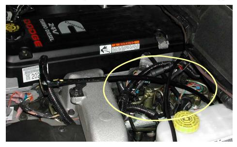
connector into the stock engine MAP sensor and the stock engine wiring harness connector into the supplied MAP sensor connector.
